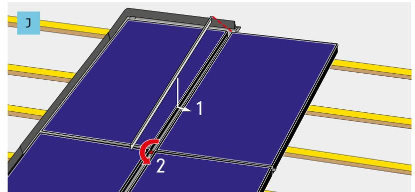
Push the joining strip (6) into the gasket in the top edge of the panel below and slide the solar panel in to engage with the joining strip and combi-brackets on two sides.
