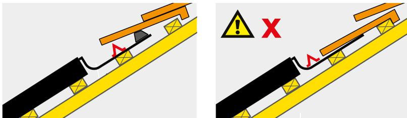
For each rafter it crosses, fix a rafter bracket (12) to the top of the top left panel and secure with two 50mm screws (20) each. You may need to add a batten above the panel to support the top flashing. Push the top flashing (5) into the panel gasket. The tile support (11) is needed for some tile types. Feed the two straps under the foam and secure the straps to a batten above.
