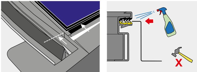
Fit the sill flashing (a) then the lower side flashing (b) to the panel. Flashings push into the rubber gasket seal in the upper slot of the panel frame. Take care to align the leading edge just above the yellow line on the gasket. If lubrication is required, use glass cleaning fluid.
