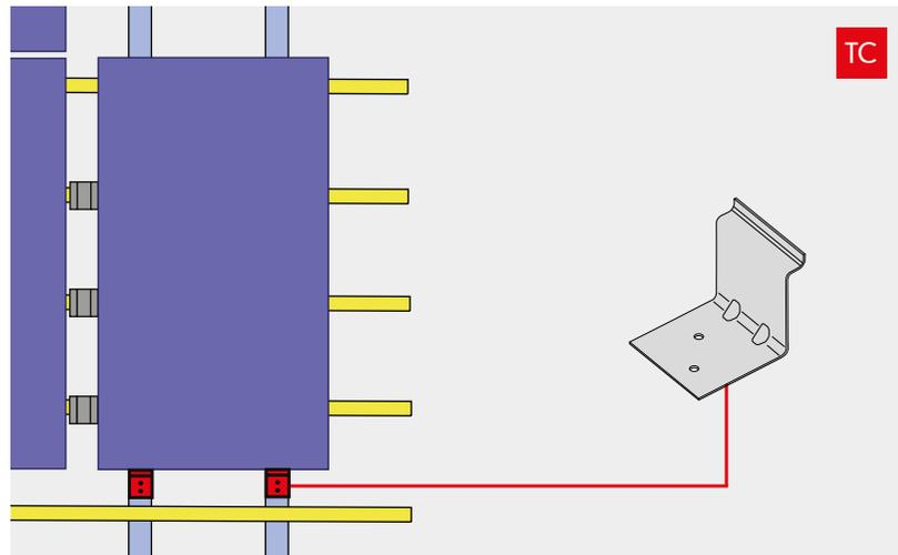
Slide the first panel of the next column sideways to engage with the combi-batten brackets. The bracket sets the gap to 30 mm. Secure the new solar panel to each rafter it crosses with rafter brackets (12) and two 50mm screws (20) each.
