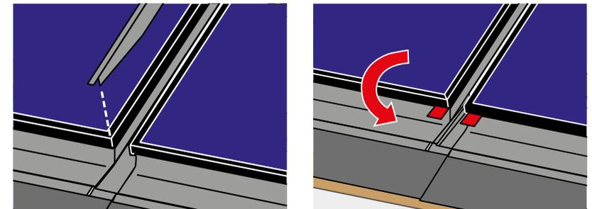
Align the bottom corner of the lower gutter covers (8) with the bottom edge of the solar panel and push the gutter covers into the gasket. Fold down the retaining tabs.
