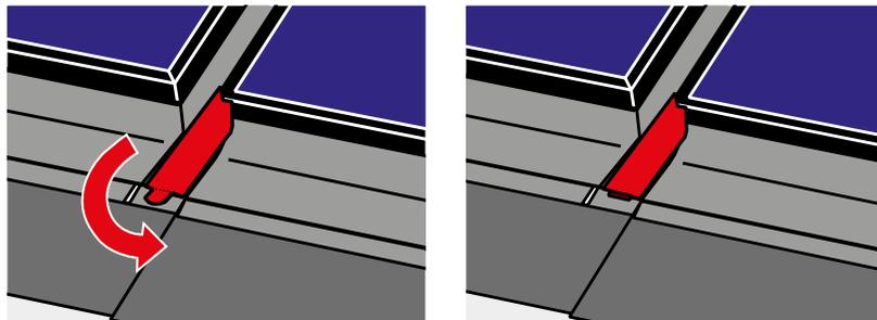
Slide the lower gutter (7) between the two solar panels from the top. Fold the tab at the bottom behind the sill flashing. Loop the gutter fixing strip (16) into the slot on top of the gutter. Fix the strip to a batten with a nail.
