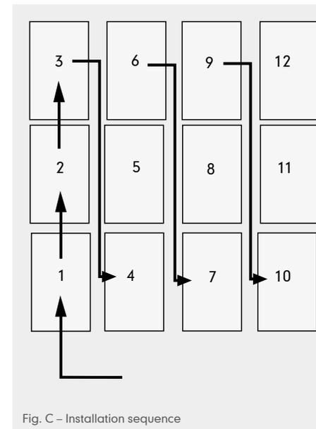
Fig. C – Installation sequence
