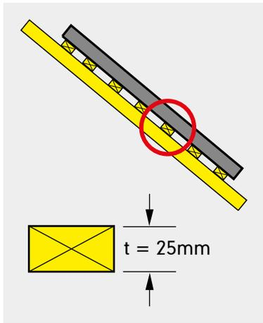
Roofing kits are provided with brackets suitable for tile battens of 25mm thickness.
