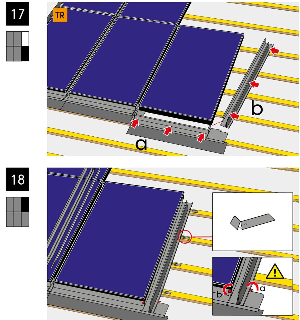
Push the sill flashing (2) into the gasket at the bottom of the solar panel. Push the lower side flashing (3) into the gasket on the right hand side of the panel.
