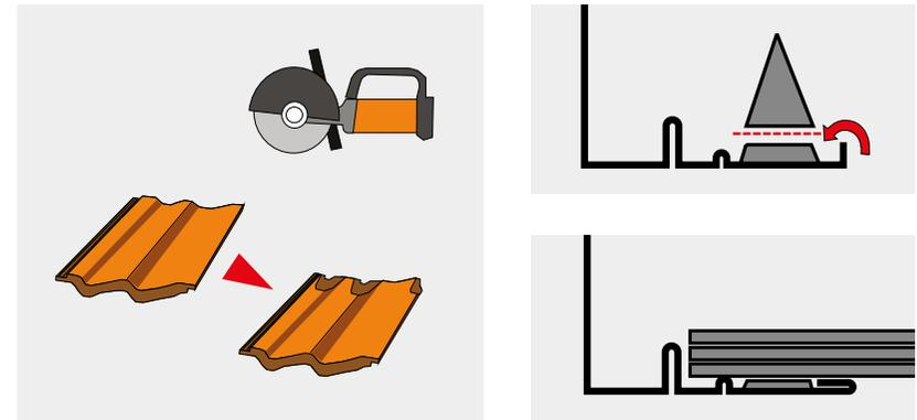
Remove the paper strip on the underside of the sill flashing and press down onto the tiles. **Ensure that the bitumen strip is well-bonded to the tiles. In some circumstances, for example a dusty tile surface, the application of a low modulus external silicone sealant will be required to achieve good adhesion.**
