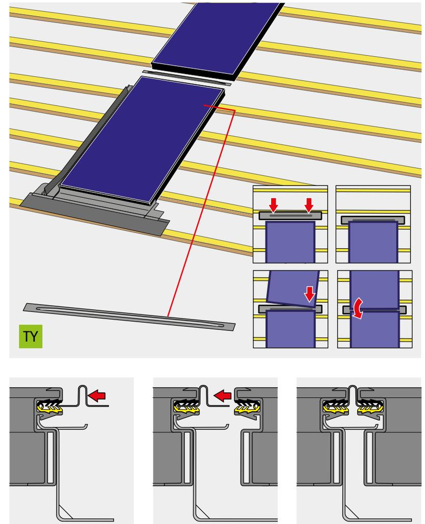
Push the joining strip (6) into the gasket on the top face of the lower solar panel. Align to the centre of the panel.
