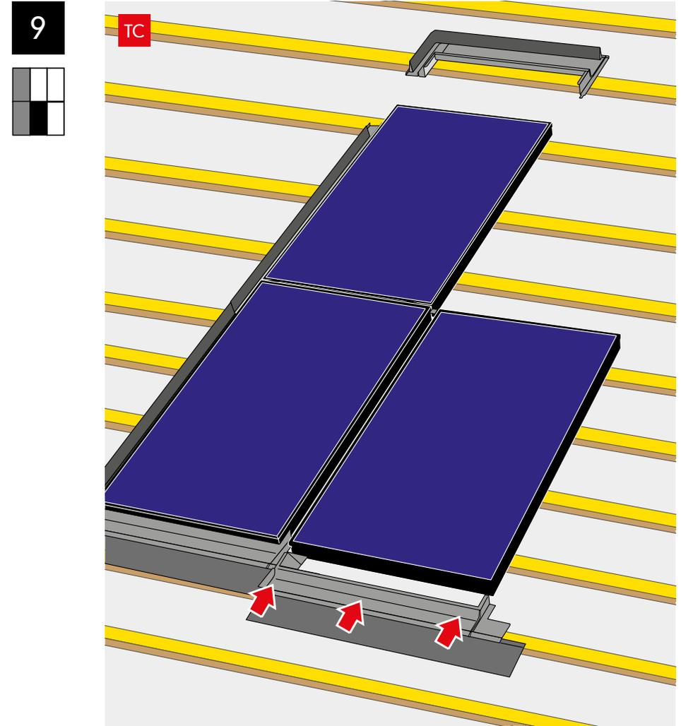
Push the sill flashing (2) into the gasket on the solar panel.
