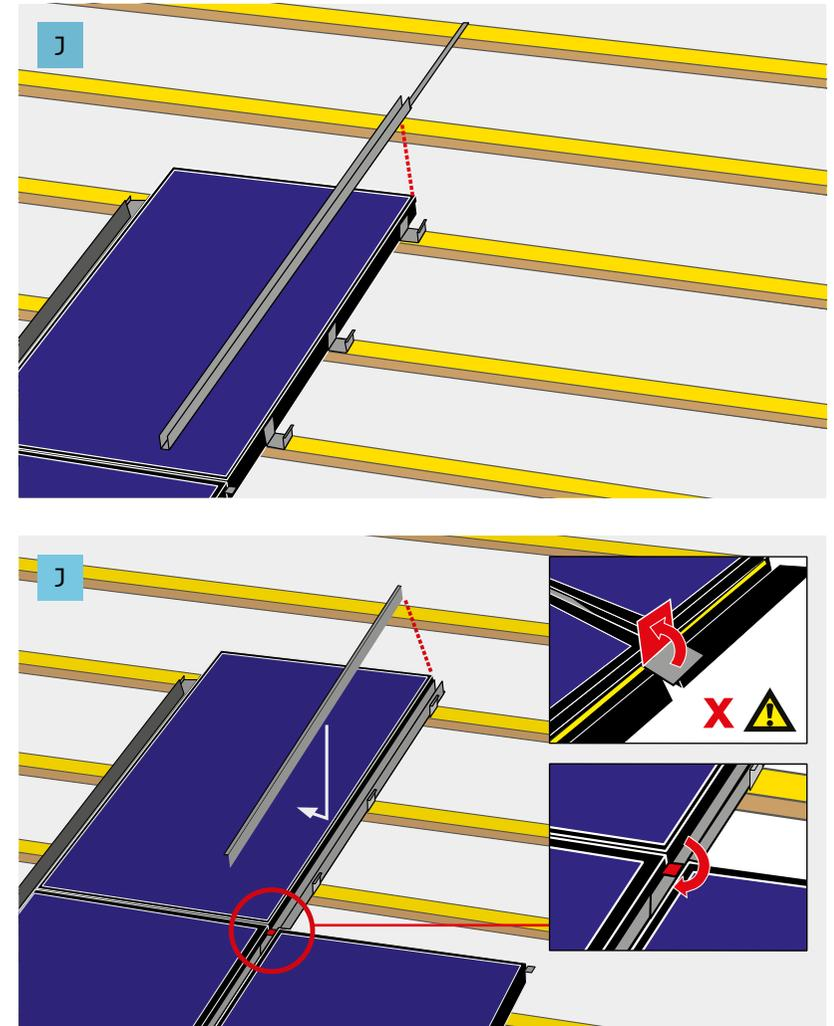
Fit the upper gutter (9) between the solar panels and nail the gutter fixing strip to a batten. Push the upper gutter cover (10) into the panel gasket. Fold the end of the joining strip down into the gutter.
