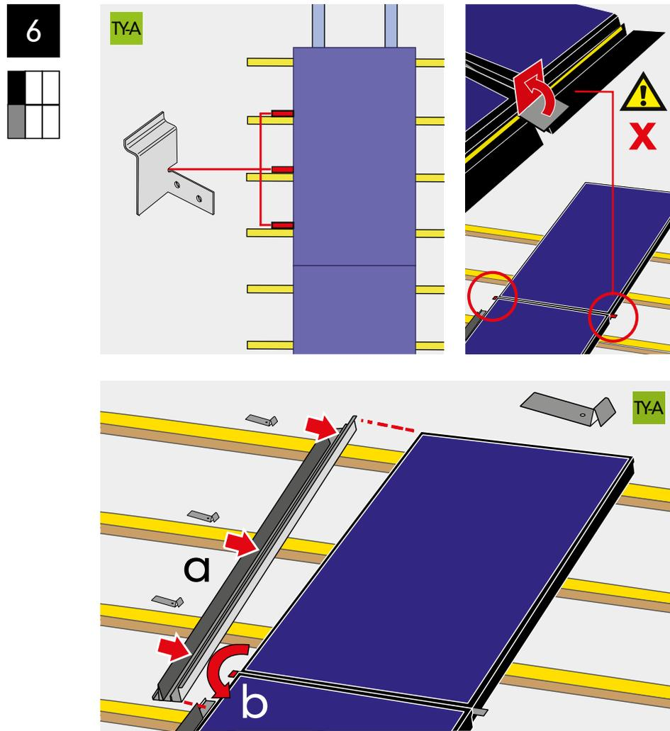
Fix the left side of the solar panel with batten brackets (14) and 25mm screws (19). Push in the upper side flashing (4) and fix the outside edge with side fixing tabs (17).
