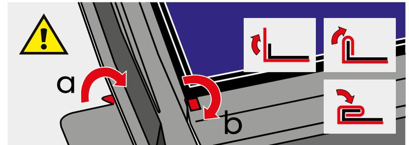
Secure the edge of the side flashing using side fixing tabs (17) and nail (18). Fold over the tab on the sill flashing (a) to grip the side flashing. Fold down the tab on the side flashing (b).
