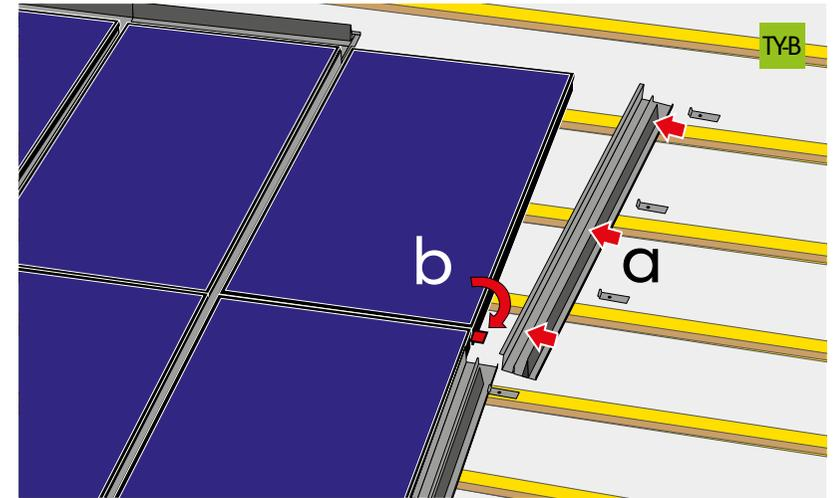
Repeat step 6 to fit batten brackets and upper side flashing
