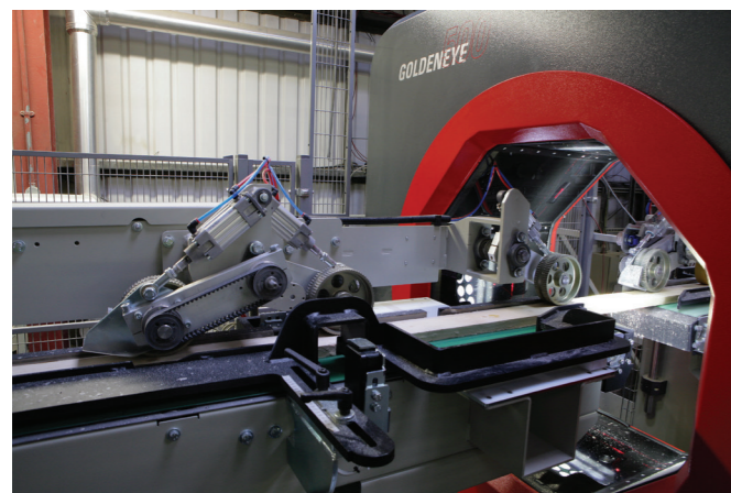
Goldeneye, roofing batten scanning line.
